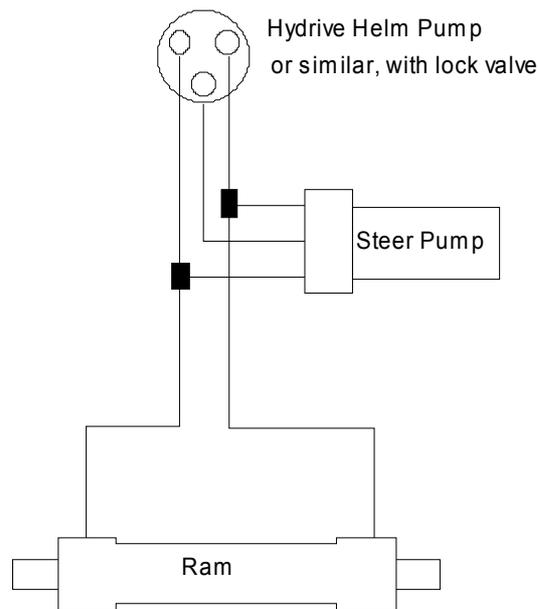
Figure 3.14 Connection to a typical two-line system
