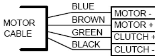
Figure 3.12. Connections to a mechanical steering drive motor.<sup>38</sup>
