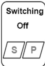
Hold down the STANDBY and PILOT keys for a second.
