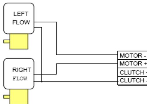
Figure 3.13 Connection to flow-control solenoids.
