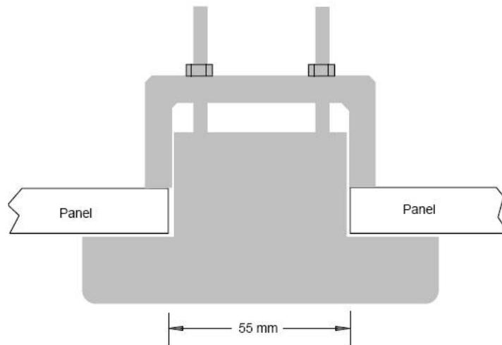
Figure 3.3 Panel mounting of the AP01 Control Head.
