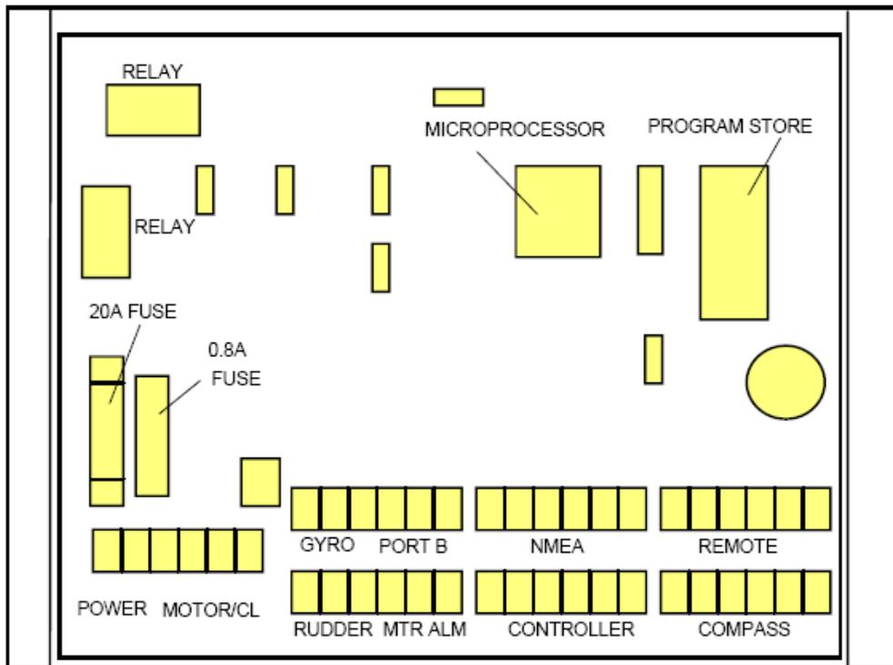
Figure 3.1 Layout of S81.01 Junction Box components and connectors.
