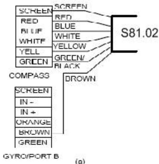
Figure 3.5. Socket connections for S81.02 fluxgate.
