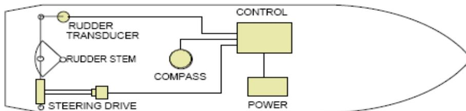
Figure 1.1 Basic components of a marine autopilot.
