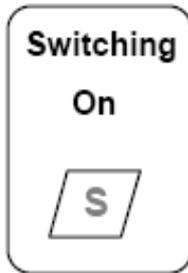
Press the STANDBY key. The system does a self-test for a few seconds and displays the version of software fitted to your autopilot. When the self-test is complete the normal STANDBY display appears and shows the current heading of the vessel.
