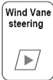
With the WIND OFF message showing, press the RIGHT ARROW key. If a wind instrument is fitted, The vessel now holds a fixed relative heading to the wind, being the one existing when the key was pressed. The relative heading is displayed on the bottom of the screen and may be adjusted via the ARROW keys. Alternatively, the system may be switched to STANDBY and a new course selected by hand steering. If data is not being received, the display shows
