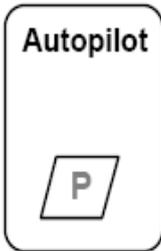
With the system in STANDBY, steer the vessel to the desired heading and press PILOT. The autopilot will now lock onto that heading and maintain it. The position of the rudder when the PILOT key was pressed is stored in memory as the effective helm centre.
