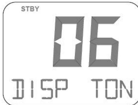
Use the arrow keys to select a displacement (weight) in ton, which is close to the actual weight of your vessel, using the arrow keys to step up or down through the range of 1 to 110 ton. Then press STANDBY.
