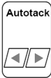
The autotack feature produces a delayed course change which is useful for single handed sailing. The tack angle is preset to 100 deg, but may be changed via the menu (See Sec 2.5). With the TACK message showing, press the LEFT or RIGHT ARROW. A 10 second countdown show on the screen and when it reaches zero, the course change starts. To cancel autotack during the countdown, press PILOT.
