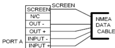
Figure 3.11 NMEA data cable connections.
