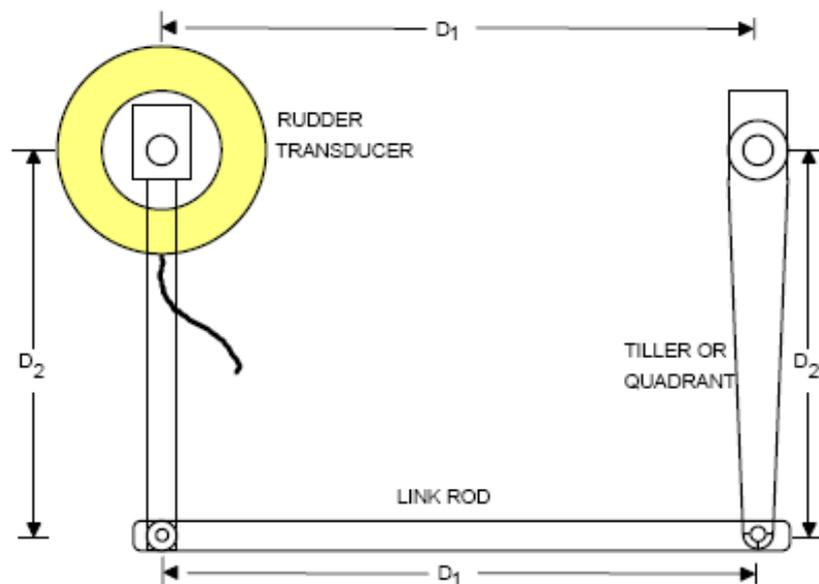
Figure 3.7 Rudder Transducer Linkage
