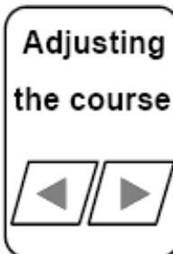
To adjust the current reference course, press either the left or right arrow key. A single press changes the course by 1 degree. Holding a key down changes the course continuously in 10 degree steps.
