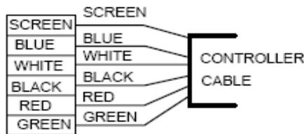
Figure 3.4 Controller cable connections.
