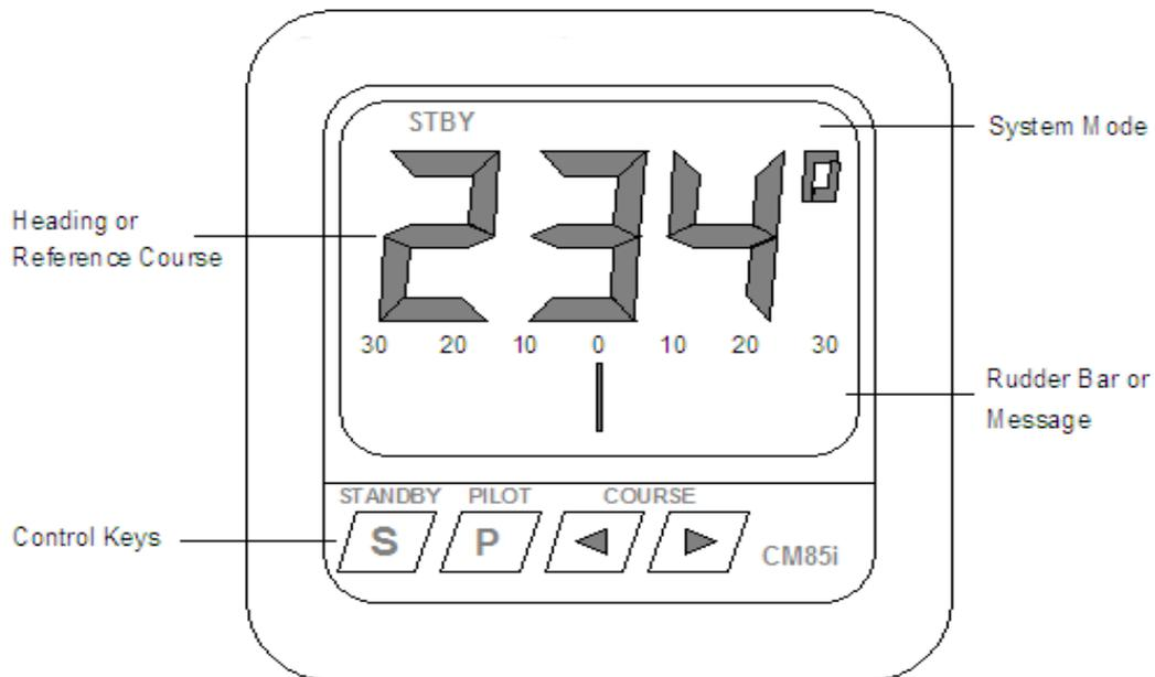
Figure 2.1 The AP01 Controller panel.
